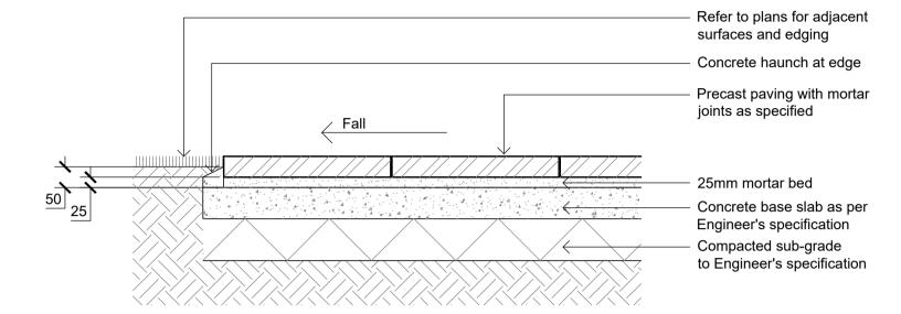
02 Unit pavers on concrete slab
